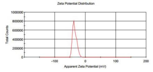
The Zeta potential of the titanium dioxide magnetic bead (thin shell) is -35.0 mV.
