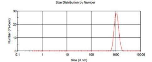
The DLS hydrodynamic size of the titanium dioxide magnetic bead (thin shell) is 1058 nm and the PDI is 0.348.
