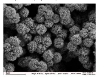
The average size of titanium dioxide magnetic beads (thin shell) is 1.20  $\mu m$ .
